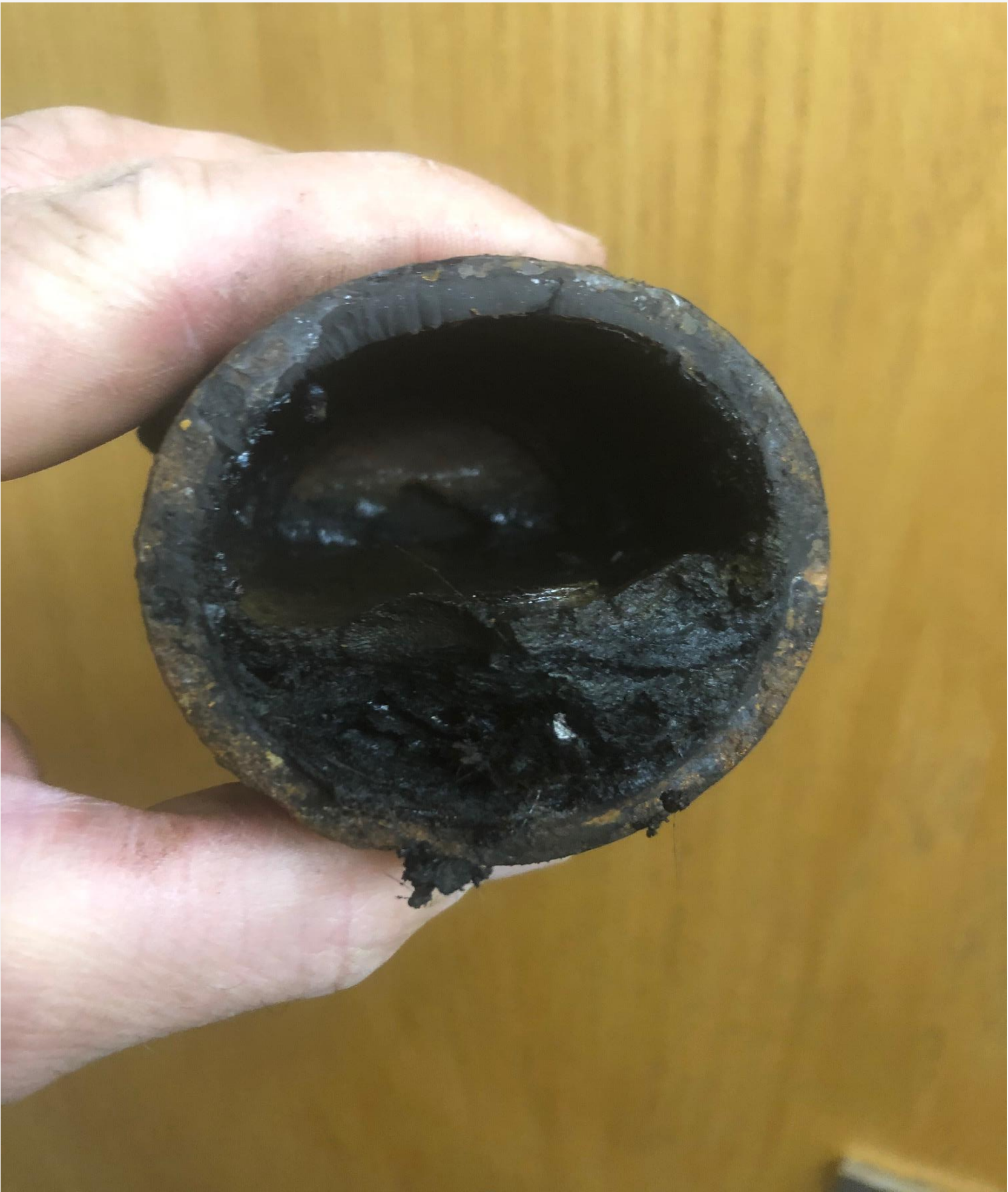
Corroded Drainpipe Throughout Building
